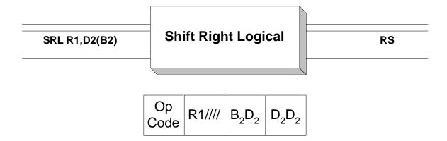
**SRL** is used to shift the 32 bits in the register specified by Operand 1 to the right. The number of bits that are shifted is indicated by Operand 2. The second operand address is **not** used to address data; instead, the base/displacement address is computed and the rightmost 6 bits are treated as a binary integer which represents the number of bits to be shifted. We will call this value the "shift factor". This leads to two distinct ways of coding the shift factor:
