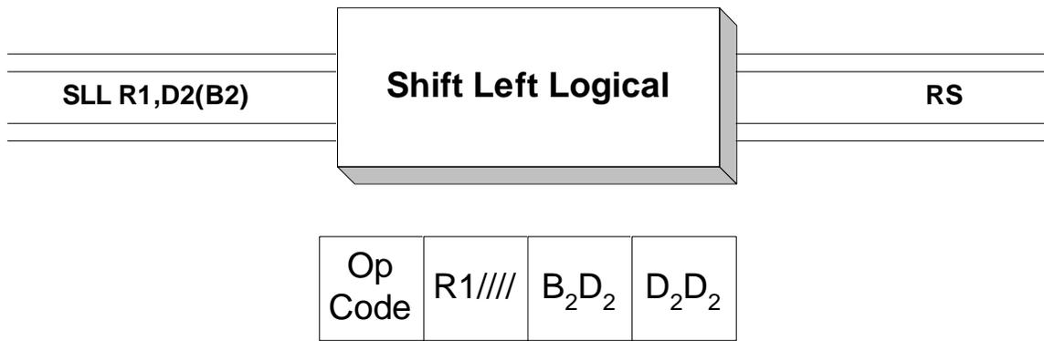
**SLL** is used to shift the 32 bits in the register specified by Operand 1 to the left. The number of bits that are shifted is indicated by Operand 2. The second operand address is **not** used to address data; instead, the base/displacement address is computed and the rightmost 6 bits are treated as a binary integer which represents the number of bits to be shifted. We will call this value the “shift factor”. This leads to two distinct ways of coding the shift factor:
