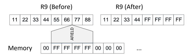
The contents of the fullword "AFIELD" are copied to the rightmost 32 bits of register 9, destroying the previous values in R9. The fullword is unchanged by this operation.
